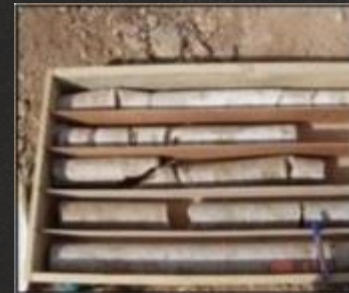
Photo: Limestone core samples from a project in Iraq.
